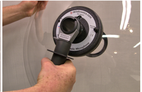
Tighten Handle clamp.
