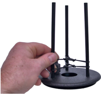
Assemble o-rings onto frame.
